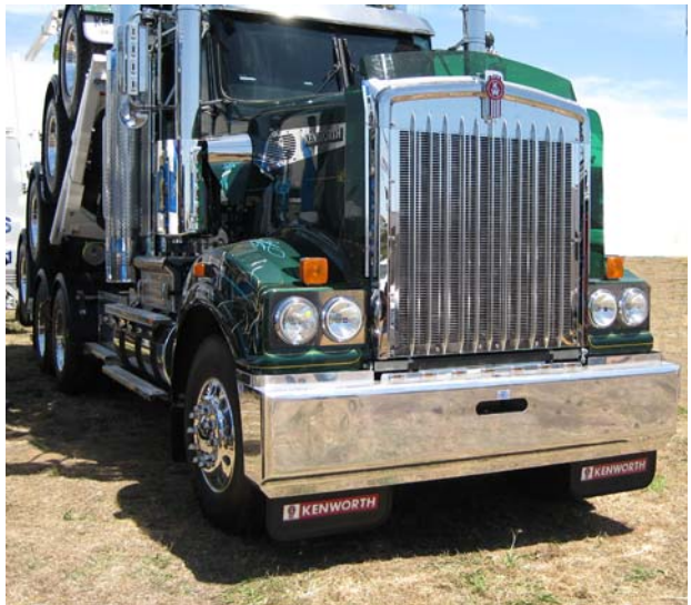
ADV7707 T904, T908, T909 "TEXAS" FUPD BUMPER with removeable TOWPIN Approval No. FUP10144/09
