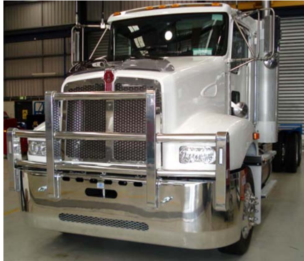
ADV7673 KEN T388 5A FUPD Bullbar Approval No. FUP10092/09 ADV7704 KEN T358/T359 5A FUPD Bullbar Approval No. FUP10092/09 NEW
